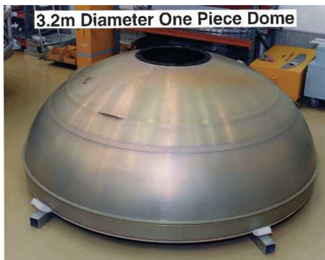
Fig. 1 One-piece dome for a cryogenic tank (2219 alloy)
